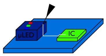
Fig. 2: Contacting of Micro LED and driver IC on pixel level by UPD printing
