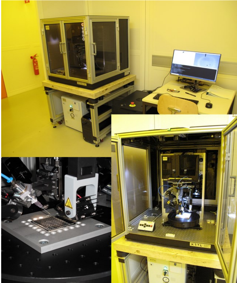
Fig. 1: XTPL® DELTA Ultra-Precise Deposition Printing System in the cleanroom of the Institute for Large Area Microelectronics
